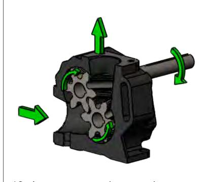
If the pump is turning as shown view above, the Front valve is controlling pressure. The rear valve can not open in this condition, as the fluid pressure is pushing against it.
