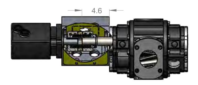
Set distance from mount face. Used for Hydraulic motors and Gear Meters.
