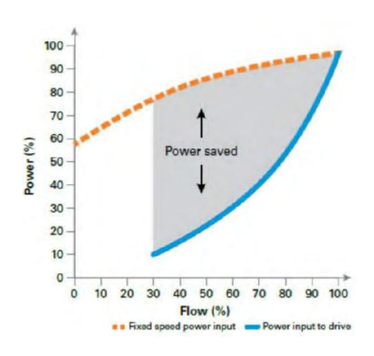
\*Fixed Speed; Not everyone will choose some type of speed control. As a cautionary measure, we advise all fixed drive systems start at a reduced speed. This should be as much as 50% below the pumps maximum. At initial start-up, this slower speed is more forgiving When conditions are not as expected. Once the issues are corrected, the motor pulley can be replaced with a larger pulley to increase speed as conditions allow.
