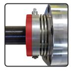
**Double Lip Seal** The main seal has a single ring in contact with the emulsion. The seal has a neighboring grease cavity which lubricates and prevents material adhesion.
